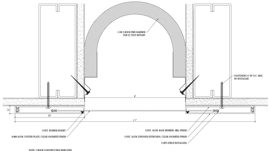
NOTE: 1 HOUR CONSTRUCTION INDICATED 2 LAYERS OF GYPSUM BOARD FOR 2 HOUR CONSTRUCTION
